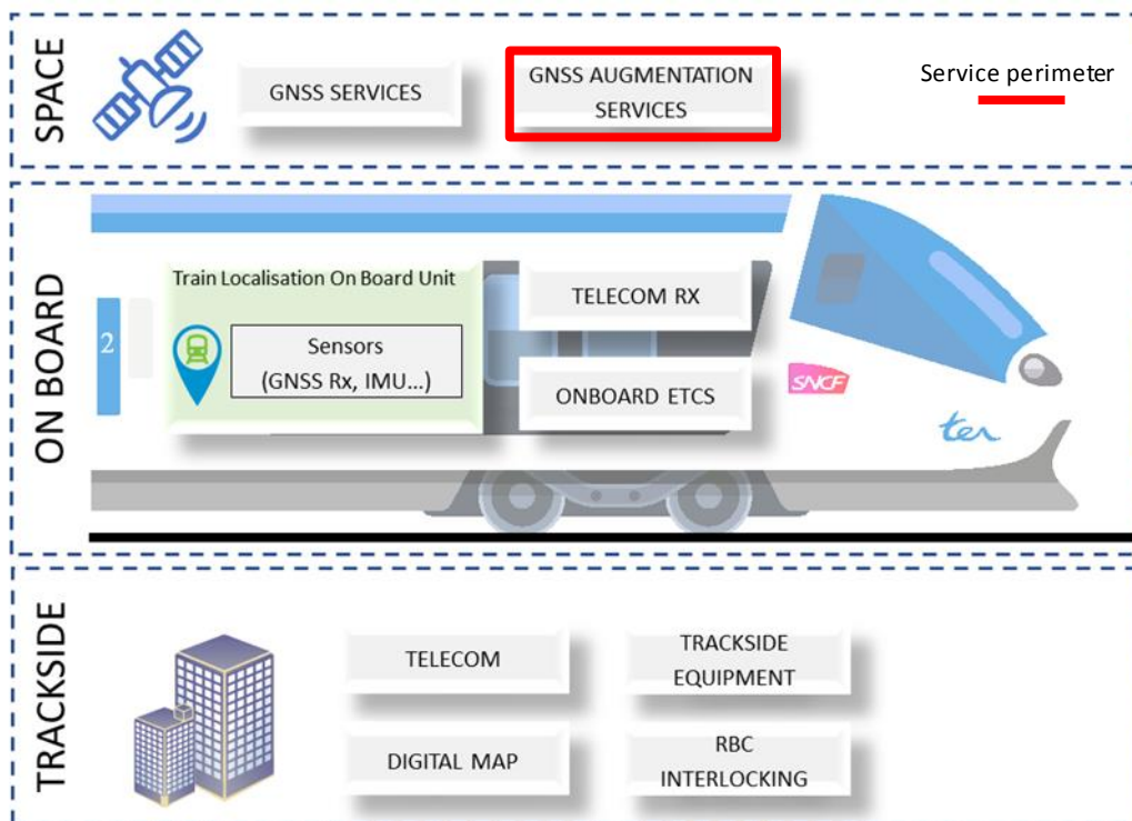
Figure 1: Scope of the GNSS Augmentation service among the 3 main contributing segments
